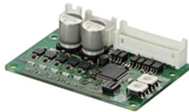
2-phase, fully digital, bipolar microstepping driver, CVD
